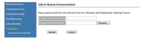
Note: - The In-Queue Announcement File must be in the following format: 8 KHz/16bit/MONO .wav or .ZIP (if you use the GXE502X IVR/System Prompt Conversion Tool).
